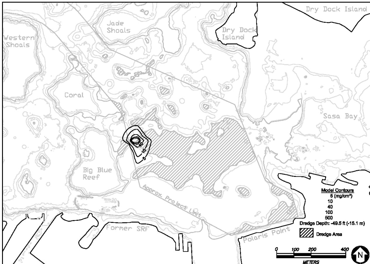
Figure 4: Sediment Deposition Contours from Sea Engineering Inc. Model Run 7B (Source: SEI 2009, Section E of this report)
