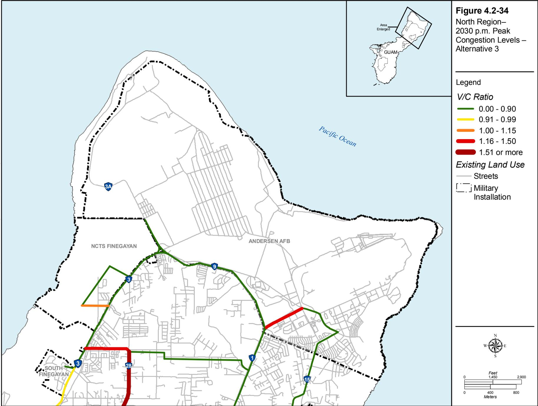
As shown in Table 4.2-14, there are three intersections and three access points with LOS F for at least one peak hour, which is considered unacceptable. The Route 1/29 intersection is operating at LOS F in the a.m. and p.m. peak hours in both 2014 and 2030.
