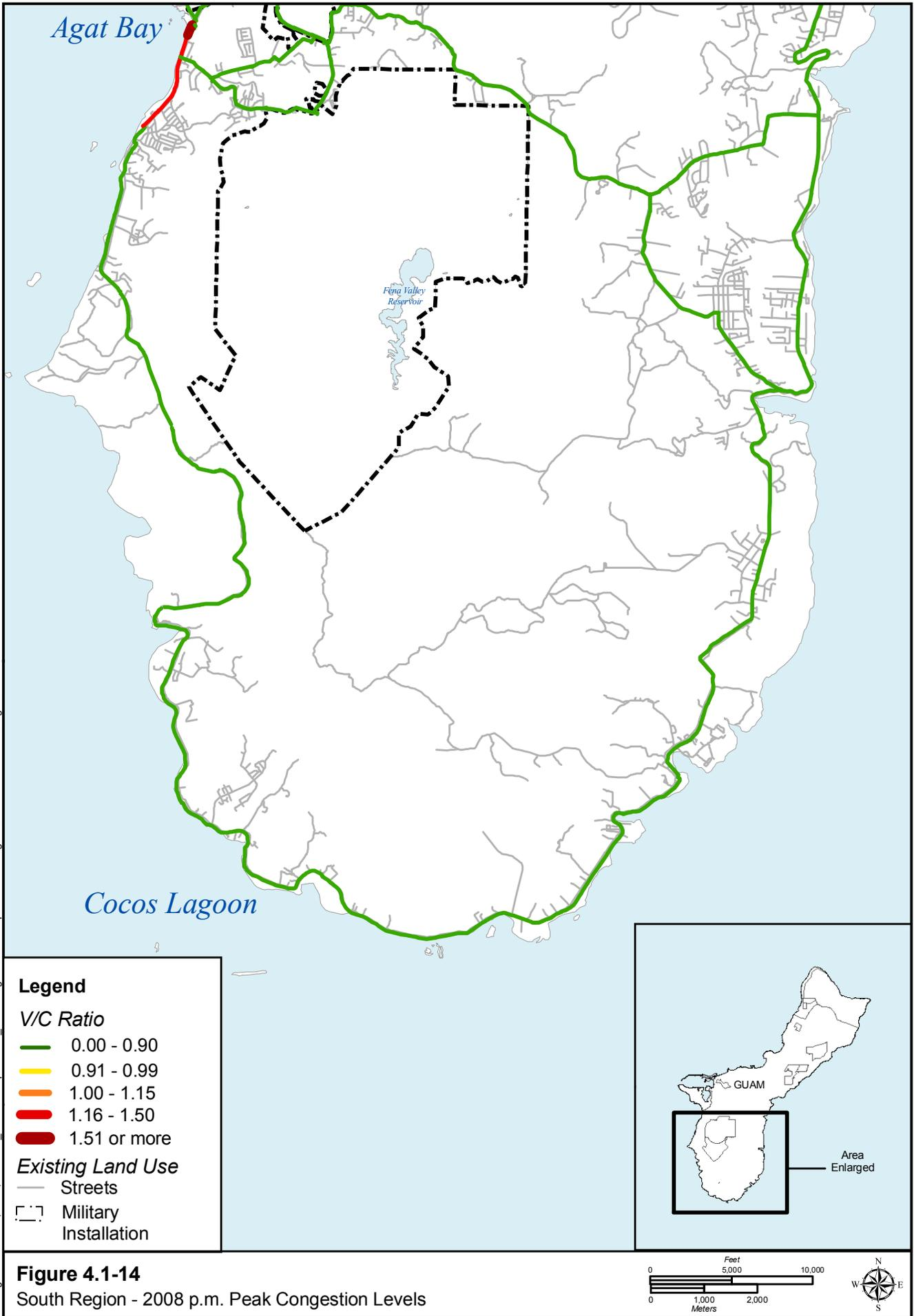
Although there are numerous intersections with capacity issues, there are not currently many roadways included in this study with a high existing V/C ratio. During both the morning and afternoon peaks, the roadways included in this area of interest are all considered not congested in both the a.m. and p.m. peak hours.
