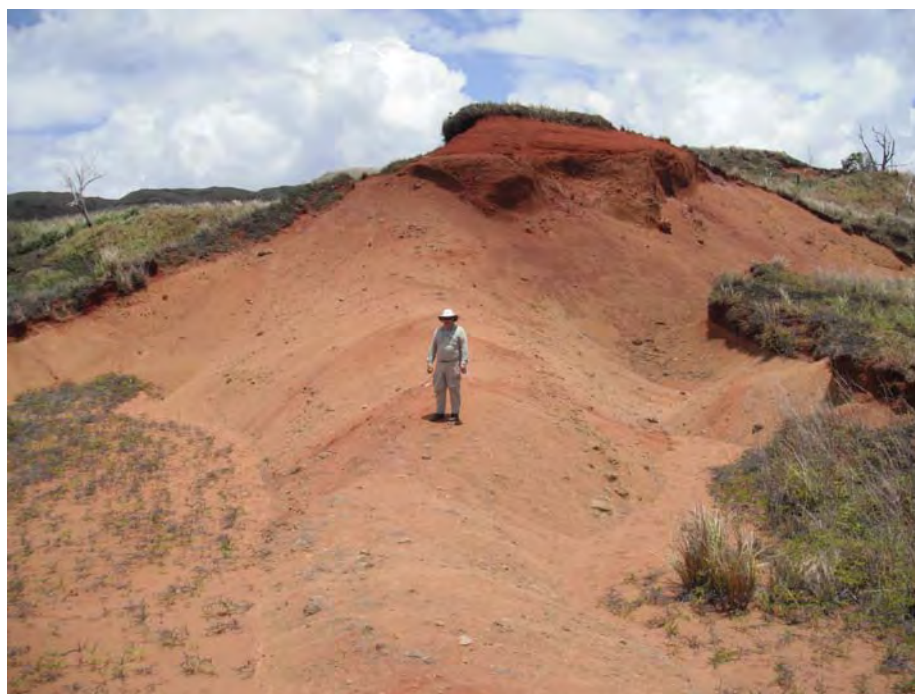
PHOTO 23 LARGE EROSIONAL AREA WITH ACTIVE GULLYING AND REMNANTS OF HEADWALL FAILURE.
